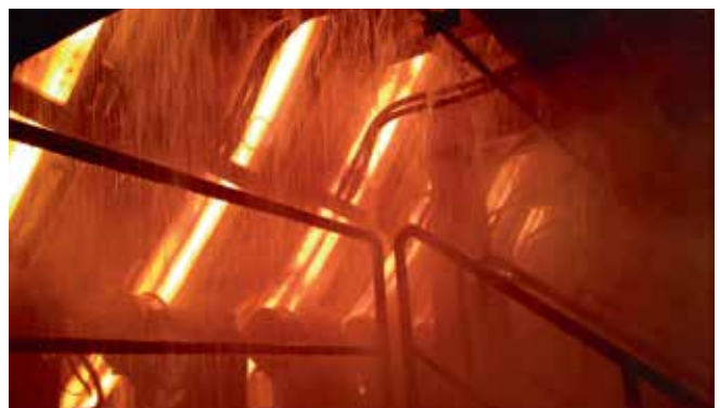
Secondary cooling zone of billet caster
