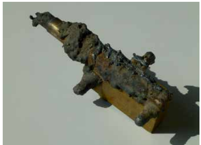
Air mist nozzle after break out of liquid steel
