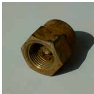
Clogged vane of a full cone nozzle
