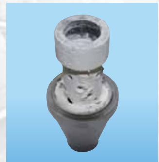
Nozzle blocked as a result of operation with lime slurry
