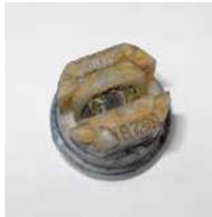
Clogged nozzle (front side)
