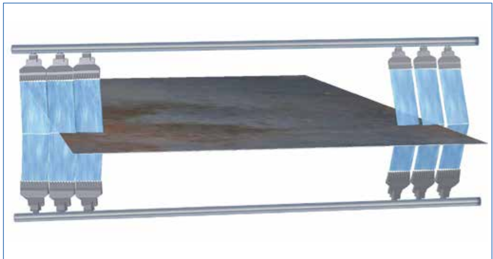
Strip edge blow-off with multi-channel nozzles for compressed air
