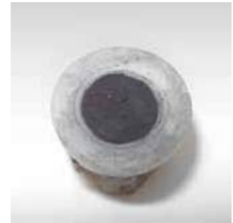
Clogged nozzle (back side)
