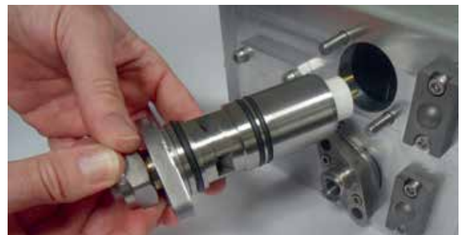
Totally serviceable from the header front
