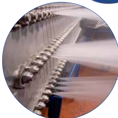
Upper selective roll coolant header
