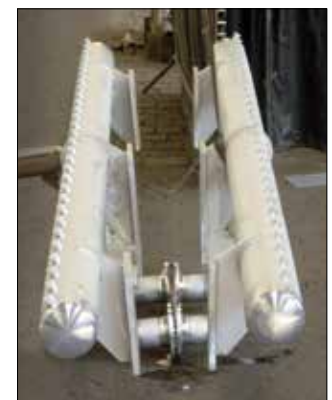
Optimized spray header designed and fabricated by Lechler
