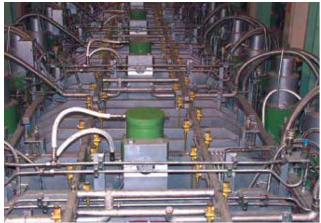
Horizontal segments with Mastercooler SMART nozzles
