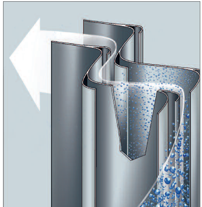
Functional principle of a horizontal separator
